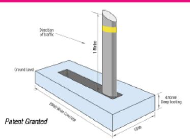
Height Above Ground: 1 metre Footing Depth: Only 470mm Options: Stainless Steel & Mild Steel Shrouds Available Still Working After Impact
