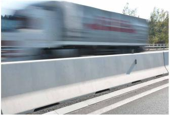
Containment level Working width Impact severity level H4b (covers H3, H2, H1, N1, T3, T2 and T1) W6 (covers W7 and W8) ASI B
