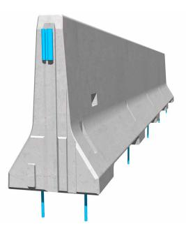
Permanent precast concrete vehicle restraint systems are used for long lasting protection on the central reservation and along the verge. Vehicles deviating from the road are retained or redirected and prevent a dangerous breakthrough onto the opposite carriageway. The highest containment level H4b offers best possible protection and even restrains an impact of a 38 t truck driving at 65 km/h (TB81 according to EN1317-2).
