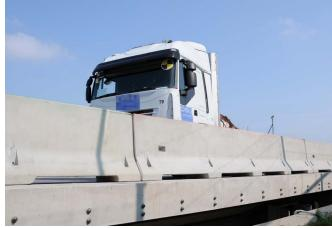
**Containment level** Working width Impact severity level H4b (covers H3, H2, H1, N1, T3, T2 and T1) W2 (covers W3, W4, W5, W6, W7 and W8) ASI B
